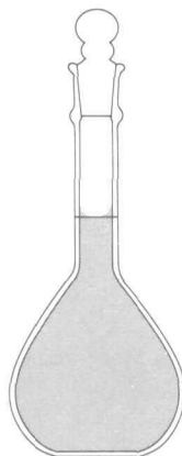
FIGURE 7-1 Volumetric flask filled to the mark with a liquid.
