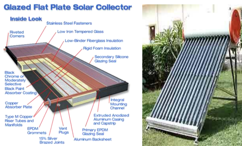
Fig.3 .Flat Plate liquid collector
