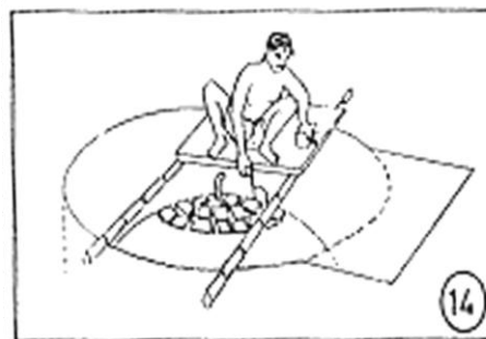
Closing of dome with bricks
