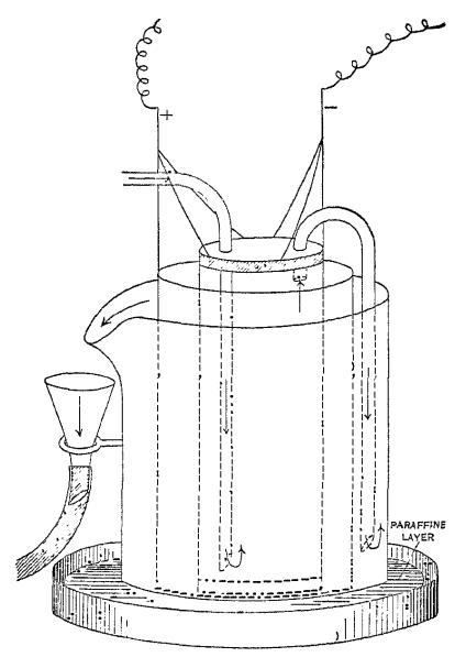
FIG. 1.—Arrangement for Cooling the Electrodes.
