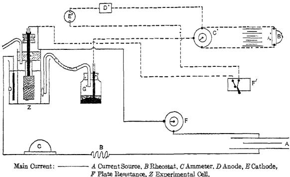
Measuring Current:..... A' Compensation Accumulators, B' Precision Voltmeter, C' Plate Resistance, D' Ballast Resistance, E' Galvanometer, F' Instantaneous Cutout, G Standard Electrode.
