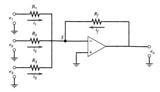
Figure 15.2.3 An adder circuit.
