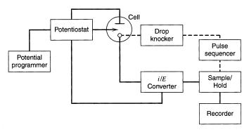
Figure 7.3.4 Schematic experimental arrangement for tast polarography. Staircase voltammetry is carried out at a stationary electrode with the same system except the drop knocker.
