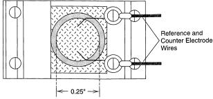
Figure 16.2.3 Cell for electrochemical STM. *Upper*: schematic diagram. *Lower*: Nanoscope III cell, top view. [Courtesy of Digital Instruments, Veeco Metrology Group].
