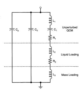
Figure 17.5.3 Equivalent circuit for a quartz crystal under mass and liquid loading. The circuit elements of the unperturbed crystal are  $L_1$ ,  $C_1$ ,  $R_1$ , and  $C_0$ . Liquid- and mass-loading adds additional elements  $L_2$ ,  $R_2$  and  $L_3$ .  $C_p$  represents any parasitic capacitance of the test fixture. [Reprinted with permission from S. J. Martin, V. E. Granstaff, and G. C. Frye, Anal. Chem., 63, 2272 (1991). Copyright 1991, American Chemical Society.]
