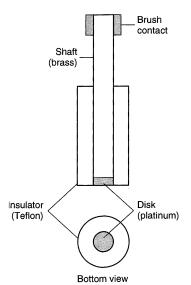
**Figure 9.3.1** Rotating disk electrode.
