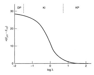
Figure 12.3.20 Variation of half-peak potential with  $\lambda$  in the ErC; case.
