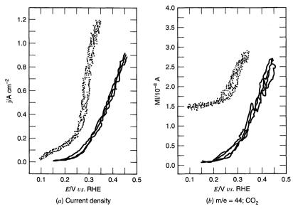
**Figure 17.3.16** Results for oxidation of formic acid (dotted curves) and methanol (solid curves) at a fuel-cell anode (Pt/Ru) with phosphoric-acid-doped polybenzimidazole polymer electrolyte, 170°C. (a) current density and (b) mass signal for CO<sub>2</sub> at a scan rate of 1 mV/s. [From M. Weber, J.-T. Wang, S. Wasmus, and R. F. Savinell, *J. Electrochem. Soc.*, **143**, L158 (1996), reprinted by permission of the publisher. The Electrochemical Society, Inc.]
