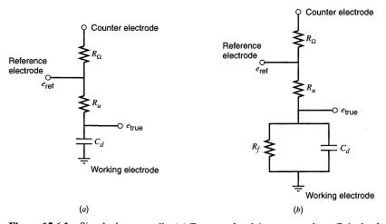
**Figure 15.6.1** Simple dummy cells. (a) For a nonfaradaic system, where  $C_d$  is the double-layer capacitance and  $R_u + R_\Omega$  is the solution resistance, with  $R_u$  being uncompensated. (b) For a system passing faradaic currents through  $R_f$ , as well as nonfaradaic ones through  $C_d$ .
