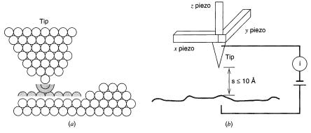
**Figure 16.2.1** (a) Representation of tunneling between tip and sample atoms. Shaded portions denote electron distributions. (b) Tip attached to three piezo elements used to position the tip and scan it across a surface.
