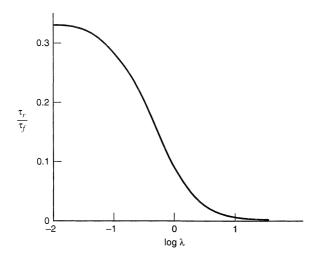
**Figure 12.3.37** Variation of  $\tau_r/\tau_f$  with  $\lambda$  for chronopotentiometry in the  $E_rC_iE_r$  reaction with  $n_1 = n_2$ . [Data from H. B. Herman and A. J. Bard, *J. Phys. Chem.*, **70**, 396 (1966).]
