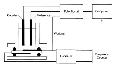
Figure 17.5.2 Schematic diagram of cell and apparatus for electrochemical QCM studies.
