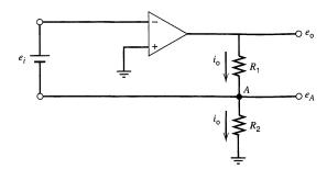
Figure 15.3.2 A circuit for controlling the potential at point A regardless of changes in  $R_1$  and  $R_2$ . Note that the feedback circuit passes through the voltage source, which is shown for simplicity as a battery.
