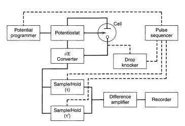
Figure 7.3.11 Schematic experimental arrangement for differential pulse polarography. For clarity, this diagram shows the functions as they would be organized in separate electronic stages in a free-standing DPP unit. In contemporary instruments, a computer performs many of the roles delineated here, including sequencing, recording of data, calculation of difference signals, and display of results.
