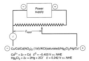
Figure 1.3.4 Schematic cell connected to an external power supply. The double slash indicates that the KCl solution contacts the Cd(NO<sub>3</sub>)<sub>2</sub> solution in such a way that there is no appreciable potential difference across the junction between the two liquids. A "salt bridge" (Section 2.3.5) is often used to achieve that condition
