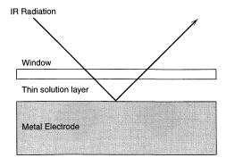
**Figure 17.2.1** Diagram of the external reflectance configuration for IR-SEC. The cell window (e.g., CaF<sub>2</sub>, Si, ZnSe) must be transparent to IR radiation and insoluble in the solution of interest.
