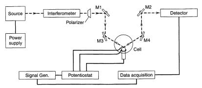
Block diagram for a SNIFTIRS instrument. The source, interferometer, detector, **Figure 17.2.4** and data acquisition usually are in a commercial FTIR instrument. [Reprinted from J. K. Foley, C. Korzeniewski, J. L. Daschbach, and S. Pons, Electroanal. Chem., 14, 309 (1986), by courtesy of Marcel Dekker, Inc.]
