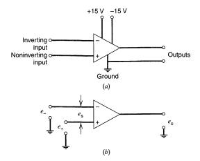
Figure 15.1.1 Schematic diagrams of operational amplifiers.
