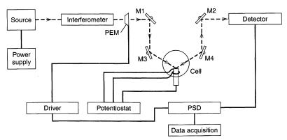
Block diagram for an IRRAS instrument with an FT spectrometer. The **Figure 17.2.5** photoelastic modulator (PEM) is a crystal, such as ZnSe, whose refractive index can be changed by application of a strain by a piezoelectric transducer, thus modulating the radiation between s- and ppolarization. [Reprinted from J. K. Foley, C. Korzeniewski, J. L. Daschbach, and S. Pons, Electroanal. Chem., 14, 309 (1986), by courtesy of Marcel Dekker, Inc.]
