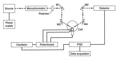
Block diagram for the instrumentation in an EMIRS experiment. The oscillator **Figure 17.2.3** varies the potential of the electrode and provides a reference signal to the phase-sensitive detector (PSD). The modulated IR signal from the detector is also fed to the PSD. [Reprinted from J. K. Foley, C. Korzeniewski, J. L. Daschbach, and S. Pons, Electroanal. Chem., 14, 309 (1986), by courtesy of Marcel Dekker, Inc.]
