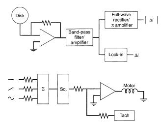
Figure 9.6.2 Schematic of speed control and disk-current processing circuitry. Only the current follower of the conventional three-electrode potentiostat that controls the disk electrode is shown.
