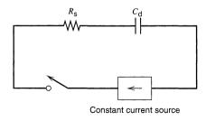
**Figure 1.2.8** Current step experiment for an *RC* circuit.
