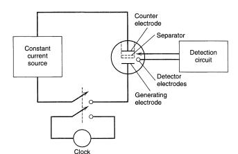
Figure 11.4.5 Apparatus for coulometric titrations.
