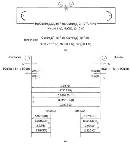
**Figure 4.3.4** Balance sheet for the system in Figure 4.3.3, but with excess NaClO<sub>4</sub> as a supporting electrolyte. (a) Cell schematic. (b) Various contributions to the current when 6e are passed in the external circuit per unit time (i = 6, n = 1).  $t_{\text{Cu(II)}} = [(2 \times 10^{-3}) \, \lambda/(2 \times 10^{-3} + 10^{-3} + 3 \times 10^{-3} + 0.2)\lambda] = 0.0097$ . For Cu(II) at the cathode,  $|i_{\text{m}}| = (1/2)(0.0097)(6) = 0.03$ ,  $i_{\text{d}} = 6 - 0.03 = 5.97$ .
