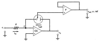
Figure 15.5.1 A simple galvanostat based on the scaler/inverter circuit.
