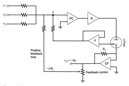
Figure 15.6.3 An adder potentiostat with positive feedback compensation.
