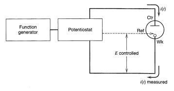
Figure 5.1.1 Experimental arrangement for controlled-potential experiments.
