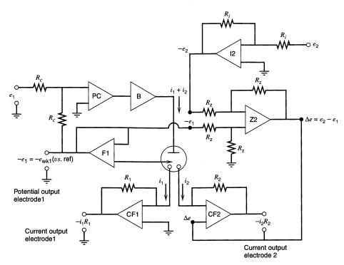
**Figure 15.4.6** A bipotentiostat based on the adder concept. On the left is essentially the system of Figure 15.4.5, which is devoted to electrode 1. On the right is a network for controlling electrode 2. For large currents at both electrodes, boosters might have to be added to CF1 and CF2.
