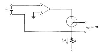
Figure 15.5.2 A galvanostat based on the circuit of Figure 15.3.3.
