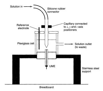
Figure 9.7.2 Schematic drawing of arrangement for wall jet or microjet electrode. [Reprinted with permission from J. V. Macpherson, S. Marcar, and P. R. Unwin, Anal. Chem., 66, 2175 (1994). Copyright 1994, American Chemical Society.]
