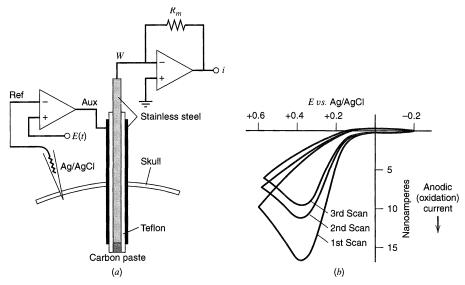
**Figure 6.6.5** Application of cyclic voltammetry to *in vivo* analysis in brain tissue. (a) Carbon paste working electrode, stainless steel auxiliary electrode (18-gauge cannula), Ag/AgCl reference electrode, and other apparatus for voltammetric measurements. (b) Cyclic voltammogram for ascorbic acid oxidation at C-paste electrode positioned in the caudate nucleus of an anesthetized rat. [From P. T. Kissinger, J. B. Hart, and R. N. Adams, Brain Res., 55, 20 (1973), with permission.]
