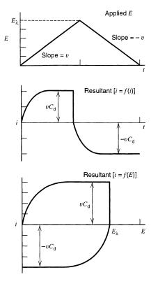
**Figure 1.2.11** Current-time and current-potential plots resulting from a cyclic linear potential sweep (or triangular wave) applied to an *RC* circuit.
