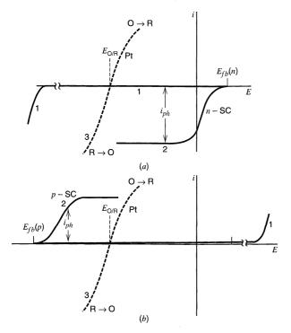
Figure 18.2.7 Current-potential curves for a solution containing couple O/R. (a) n-type semiconductor in the dark (curve 1) and under irradiation (curve 2). (b) p-type semiconductor in the dark (curve 1) and under irradiation (curve 2). For both (a) and (b), curve 3 is the i-E curve at a platinum electrode.
