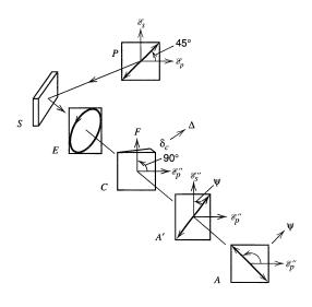
Figure 17.1.13 Schematic layout of one type of ellipsometer. Linearly polarized light (P) is incident on the sample (S). Reflection produces elliptic polarization (E), which is restored to linear polarization (A') by the compensator (C). The analyzer (A) is adjusted to achieve extinction. [From R. H. Muller, Adv. Electrochem. Electrochem. Engr., 9, 167 (1973), with permission.]
