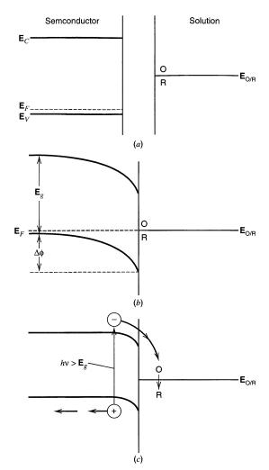
Figure 18.2.8 Formation of the junction between a p-type semiconductor and a solution containing a redox couple O/R. (a) Before contact in the dark. (b) After contact in the dark and electrostatic equilibration. (c) Junction under irradiation.
