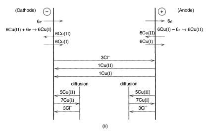
**Figure 4.3.3** Balance sheet for electrolysis of the Cu(II), Cu(I), NH<sub>3</sub> system. (a) Cell schematic. (b) Various contributions to the current when 6e are passed in the external circuit per unit time; i = 6, n = 1. For Cu(II) at the cathode,  $|i_{\rm m}| = (1/2)(1/3)(6) = 1$  (equation 4.3.3),  $i_{\rm d} = 6 - 1 = 5$ (equation 4.3.4). For Cu(I) at the anode,  $|i_m| = (1/1)(1/6)(6) = 1$ ,  $i_d = 6 + 1 = 7$ .
