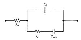
Figure 14.3.18 Equivalent circuit for an electroactive monolayer.  $R_{\Omega}$  = solution resistance,  $C_{\rm d}$  = double-layer capacitance,  $R_{\rm ct}$  = charge-transfer resistance, and  $C_{\rm ads}$  = capacitance of the adsorbed layer.
