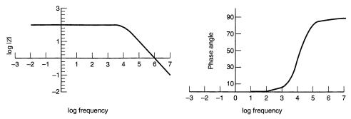
**Figure 10.1.10** Bode plots for a parallel RC circuit with  $R = 100 \Omega$  and  $C = 1 \mu F$ .
