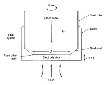
Figure 9.6.4 Schematic diagram of the apparatus employed for temperature modulation of the RDE. The laser pulse irradiates a disk electrode coated with an absorptive layer. [Reprinted with permission from J. L. Valdes, and B. Miller, *J. Phys. Chem.* 92, 525 (1988). Copyright 1988, American Chemical Society.]
