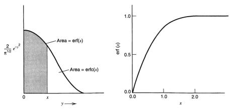
**Figure A.3.1** Definition and behavior of erf(x) and erfc(x).
