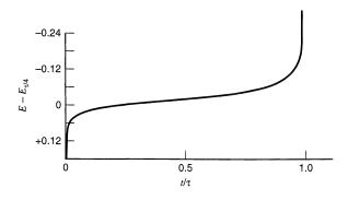
**Figure 8.2.2** Theoretical chronopotentiogram for a nernstian electrode process.
