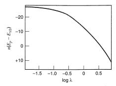
Figure 12.3.11 Variation of peak potential as a function of  $\lambda$  for the  $E_rC_i$  case. [Reprinted with permission from R. S. Nicholson and I. Shain, Anal. Chem., 36, 706 (1964). Copyright 1964, American Chemical Society.]
