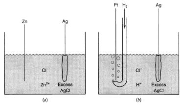
**Figure 1.1.1** Typical electrochemical cells. (a) Zn metal and Ag wire covered with AgCl immersed in a  $ZnCl_2$  solution. (b) Pt wire in a stream of  $H_2$  and Ag wire covered with AgCl in HCl solution.
