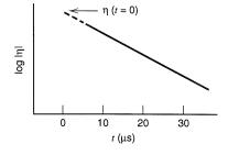
**Figure 8.7.3** Typical coulostatic relaxation curves for a totally irreversible reaction.
