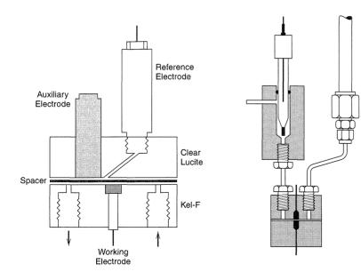
Figure 11.6.6 Thin-layer LC detector cells. Left: Cell with auxiliary and reference electrodes in thin-layer portion downstream from working electrode. Reprinted from J. A. Wise. W. R. Heineman and P. T. Kissinger, Anal. Chim. Acta, 172, 1 (1985), with permission from Elsevier Science.] Right: Cell with facing working and auxiliary electrodes and reference electrode downstream in flow channel. [Courtesy of Bioanalytical Systems, Inc.1
