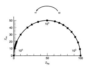
**Figure 10.1.11** Nyquist plot for a parallel *RC* circuit with  $R=100~\Omega$  and  $C=1~\mu F$ .
