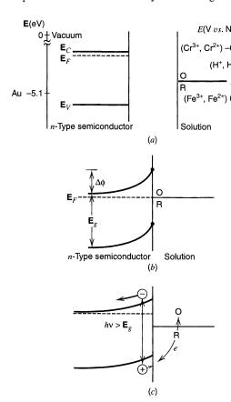
Figure 18.2.5 The formation of a junction between an n-type semiconductor and a solution containing a redox couple O/R. (a) Before contact in the dark. Typical values for energy levels shown referenced to NHE  $(E^0)$ and to vacuum (E). (b) After contact in the dark and electrostatic equilibration. (c) Junction under irradiation. [From A. J. Bard, J. Photochem., 10, 59 (1979), with permission. Adapted to show current best values for the absolute scale.]
