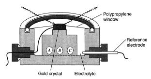
**Figure 17.6.2** Cell design for X-ray diffraction experiments with a single-crystal gold electrode. A thin layer of solution is held between the polypropylene window and the electrode. The window is held in place by an O-ring that clamps it to the Kel-F cell body. *A* and *C* are electrolyte ports and *B* is the counter electrode. [Reprinted from J. McBreen, in "Physical Electrochemistry," I. Rubinstein, Ed., Marcel Dekker, New York, 1995, Chap. 8, by courtesy of Marcel Dekker, Inc.]
