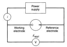
Figure 1.3.9 Two-electrode cell.
