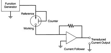
Figure 15.7.2 Alternative configuration for use with an ultramicroelectrode. The function generator produces the desired waveform and controls  $e_{ref}$  vs. ground, which is  $-E_{wk}$  vs. the reference electrode. The current at the working electrode is transduced to a voltage using a current follower in the usual manner.
