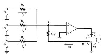
**Figure 15.4.4** A basic adder potentiostat.
