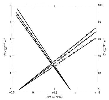
Figure 18.5.2 Mott-Schottky plots for n- and p-type InP, (111) face. Electrolyte composition: 1 M KCl + 0.01 M HCl, n-type: ( $\bigcirc$ ) 200 Hz, ( $\square$ ) 2500 Hz, ( $\Delta$ ) 20,000 Hz; p-type: ( $\bigcirc$ ) 200 Hz, ( $\square$ ) 2500 Hz, ( $\triangle$ ) 20,000 Hz. The vertical axis to the left applies to p-type, the one to the right to n-type. [From A. M. Van Wezemael, W. H. Laftere, F. Cardon, and W. P. Gomes, J. Electroanal. Chem., 87, 105 (1978), with permission.]
