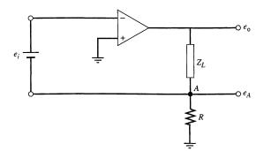
**Figure 15.3.3** A circuit for controlling the current through an arbitrary load,  $Z_L$ .
