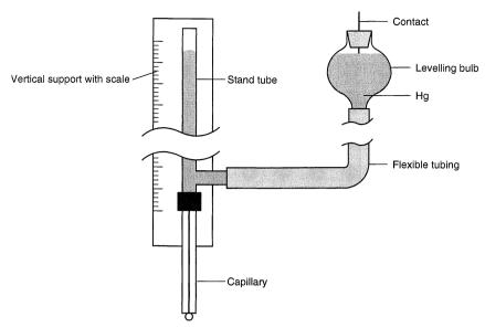
Figure 7.1.1 A dropping mercury electrode.
