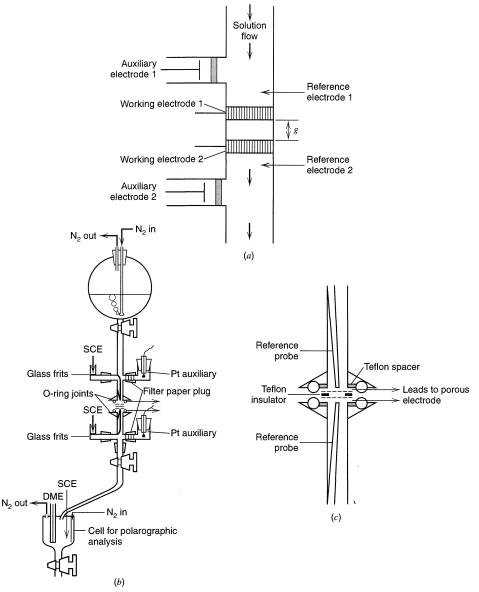
**Figure 11.6.4** (a) Schematic representation of a dual-electrode flow cell. (b) Actual complete dual-electrode flow cell assembly. Solution flows by gravity from upper reservoir. For greater clarity, the "O-ring joint" portion of the cell with the dual working electrodes is shown in exploded form. A close-up view of this portion with the porous silver electrodes is shown in (c). [From J. V. Kenkel and A. J. Bard, *J. Electroanal. Chem.*, **54**, 47 (1974), with permission.]
