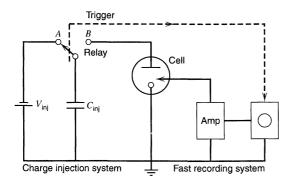
**Figure 8.7.1** Circuit for charge-step or coulostatic method. In practice, the cell may be held initially at a potential  $E_{\rm eq}$  by means of a potentiostat that is disconnected immediately before the charge injection.
