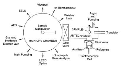
**Figure 17.3.3** Schematic diagram of apparatus that allows electrochemical preparation of sample in an antechamber under argon and then direct transfer into a UHV chamber for surface spectroscopic examination. [Reprinted from A. T. Hubbard, E. Y. Cao, and D. A. Stern in "Physical Electrochemistry," I. Rubinstein, Ed., Marcel Dekker, New York, 1995, Chap. 10, by courtesy of Marcel Dekker, Inc..]
