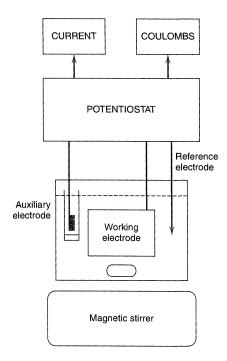
**Figure 11.3.5** Block diagram of typical controlled-potential coulometry apparatus.
