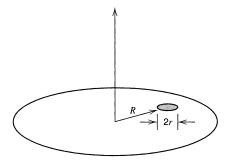
Figure 9.3.12 A rotating disk electrode where the electrode, with radius r, is offset from the axis of rotation by a distance R.
