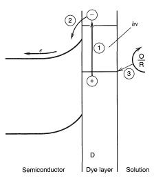
Figure 18.2.10 Dye sensitization of a photoprocess at a semiconductor electrode. For example, n-ZnO/rose bengal/I $^-$ /Pt (75).
