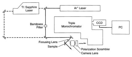
Block diagram of Raman spectrometer with a choice of laser excitation and detection with a charge-coupled device (CCD). [Reprinted with permission from J. E. Pemberton in "The Handbook of Surface Imaging and Visualization," A. T. Hubbard, Ed., CRC, Boca Raton, FL, 1995, p. 647. Copyright CRC Press, Inc., Boca Raton, FL.]
