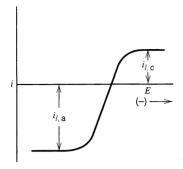
Figure 1.4.3 Current-potential curve for a nernstian system involving two soluble species with both forms initially present.
