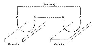
**Figure 5.9.2** Schematic representation of two microband electrodes operating in the generator-collector mode.
