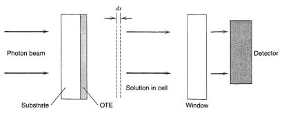
**Figure 17.1.1** Schematic view of the experimental arrangement for transmission spectroelectrochemistry.
