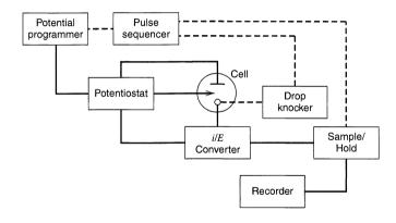
Figure 7.3.7 Schematic experimental arrangement for normal pulse polarography.
