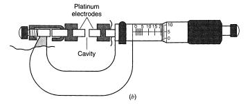
Figure 11.7.1 (a) Schematic diagram of a single-electrode thin-layer cell. (b) Micrometer, twin-electrode thin-layer cell with adjustable solution layer thickness.
