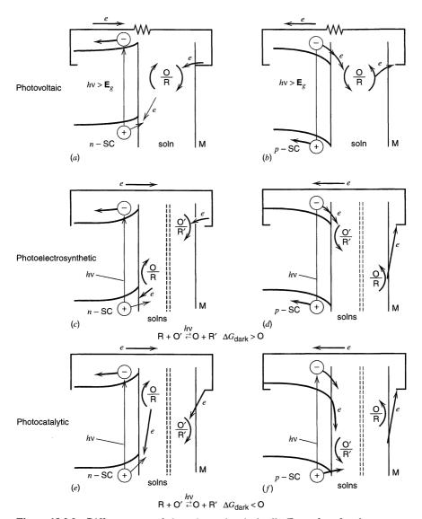
Different types of photoelectrochemical cells. Examples of each type are:
