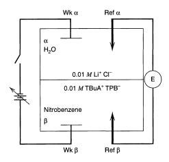
Figure 6.8.1 Schematic diagram for the apparatus for cyclic voltammetry at the ITIES between water and nitrobenzene. Ref  $\alpha$  and Ref  $\beta$ are reference electrodes, Wk  $\alpha$  and Wk  $\beta$  are metal working electrodes.
