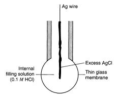
Figure 2.4.1 A typical glass electrode.
