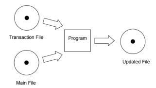
The picture shows the main file and the transaction file as input to a program. The output is a new, updated main file. The previous version of the file can be kept as backup.
