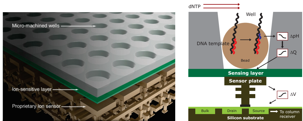
Figure 12.44 Ion Torrent technology- Sensor, well and chip architecture. An image of a well, a bead containing DNA template, and the underlying sensor and electronics. Cross section view of a single well that houses ion sphere particles with a clonal amplified DNA template. A hydrogen ion (proton) is released when a nucleotide is incorporated by DNA polymerase. The proton is then detected by the sensing layer due to the change of pH, therefore translating the chemical signal to a digital input.
