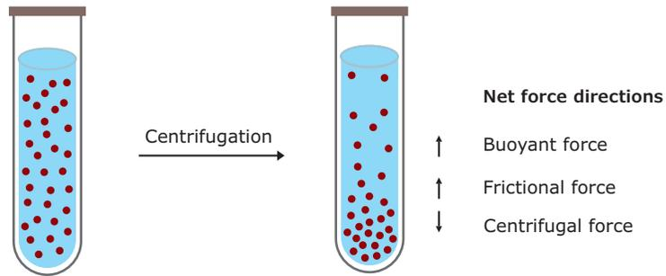
**Figure 5.1** Direction of different forces and distribution of solute particles during centrifugation.
