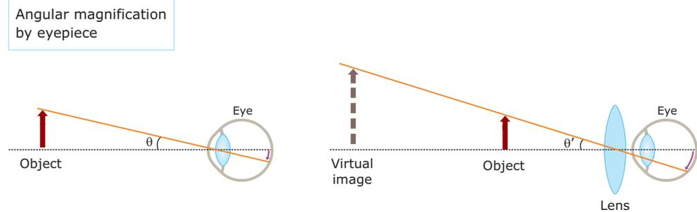
$$\text{Angular magnification} = \frac{\text{Angle subtended by image } (\theta')}{\text{Angle subtended by object } (\theta)}$$
