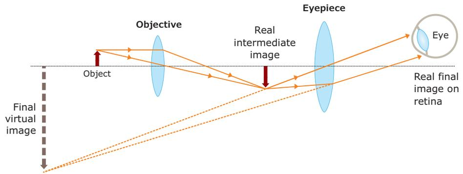
**Figure 6.1** Compound microscope and the ray diagram for image formation. It consists of two converging lenses arranged coaxially. The one facing the object is called the objective and the other close to eye is called the eyepiece.
