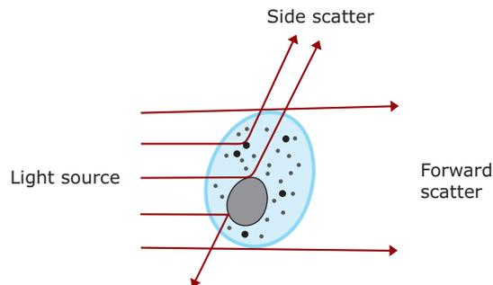
**Figure 7.2** Diagram of forward and side scatter. The amount of light scattered in a forward direction is an indicator of the relative size of a cell. This is referred to as *forward scatter*. Likewise, light scattered at higher angles gives rise to information about internal complexity and granularity of a cell, such as cytoplasmic granules, multi-lobed nucleus, cytoplasmic vacuoles, etc. This is referred to as *side scatter*.
