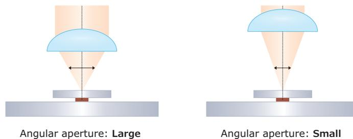
**Figure 6.4** Angular aperture and working distance. The higher value of the one-half angular aperture ( $\alpha$ ) can be obtained by shortening the distance between the objective lens and the specimen.
