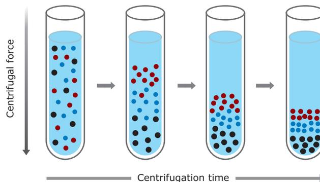
**Figure 5.3** Differential centrifugation separates particles based on differences in sedimentation rate, which reflect differences in size or density. Particles which are large or dense sediment rapidly, those that are intermediate in size or density sediment less rapidly, and the smallest or least dense particles sediment very slowly. Eventually, all of the particles reach the bottom of the tube.
