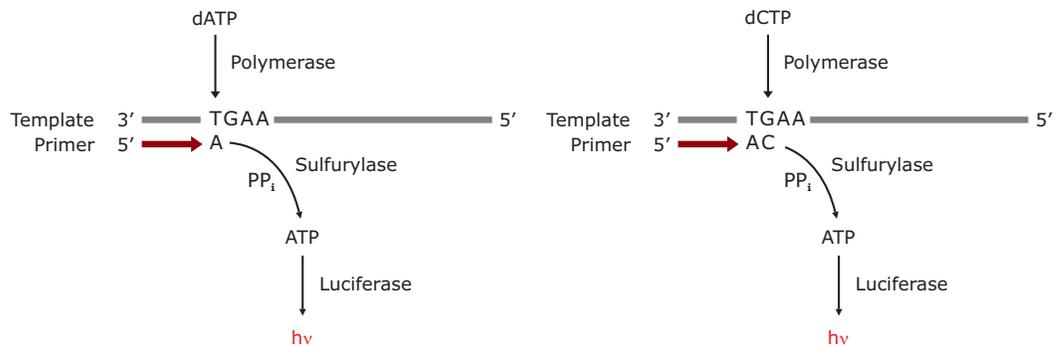
**Figure 12.43** Schematic representation of the pyrosequencing enzyme system. If the added dNTP forms a base pair with the template, DNA polymerase incorporates it into the growing DNA strand and pyrophosphate is released. ATP sulfurylase converts the  $PP_i$  into ATP which serves as substrate for the light producing enzyme luciferase. The produced light is detected as evidence of that nucleotide incorporation has taken place.
