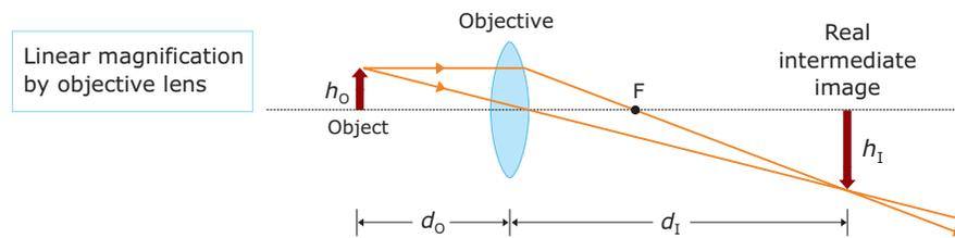
$$\text{Linear magnification} = \frac{\text{Image size}}{\text{Object size}} = \frac{h_i}{h_o} = \frac{d_i}{d_o}$$
