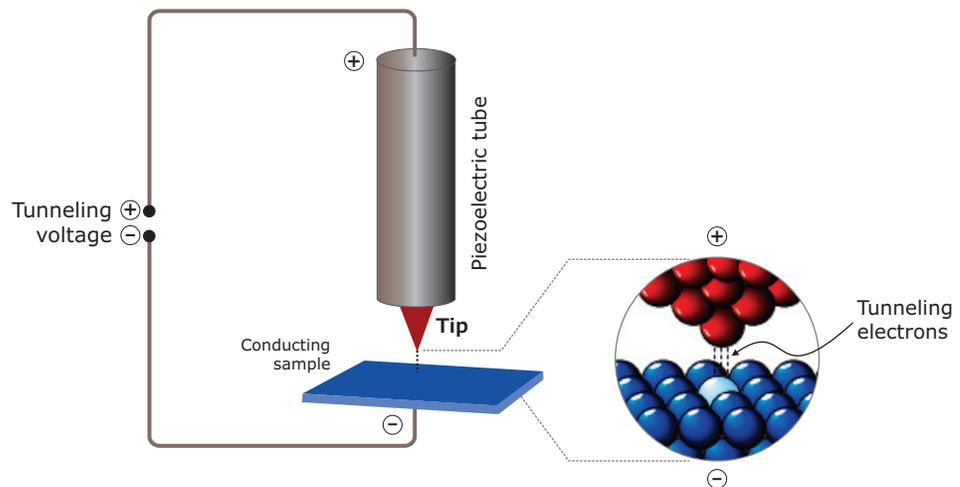
**Figure 6.15** The metal probe tip and the sample are both connected to a voltage supply. The sample is scanned by a very fine metallic probe tip mounted on a piezoelectric tube. A tunnelling current starts to flow when the tip is close to the sample. This feeble tunneling current is amplified and measured.
