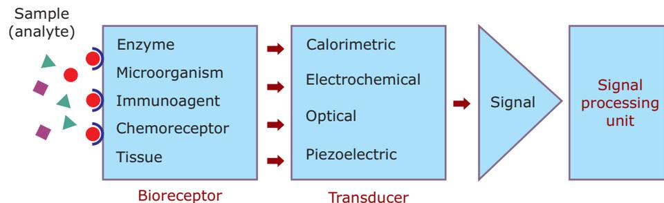
**Figure 12.45** Schematic diagram showing the main components of a biosensor. The bioreceptor – interacts with the specific analyte of interest to produce signal; the transducer – transforms the signal resulting from the interaction of the analyte with the bioreceptor into another signal (i.e. transduces) that can be more easily measured and quantified; and signal processing unit – converts the signal into a workable form (amplified, processed and displayed).
