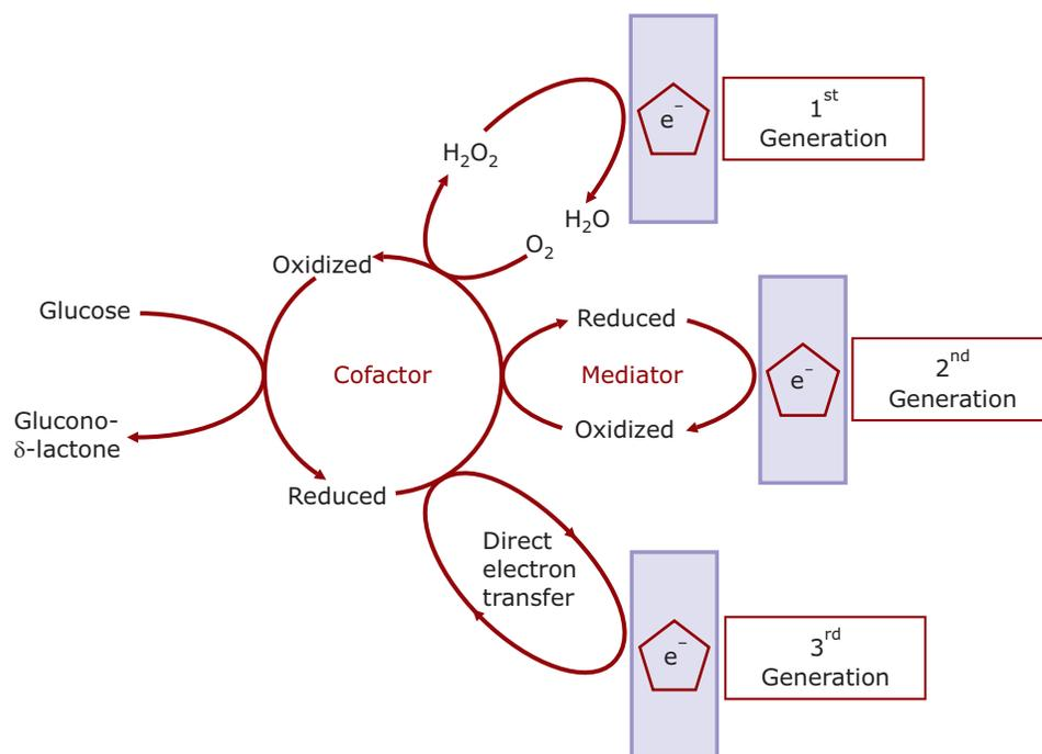
**Figure 12.47** The evolution from 1<sup>st</sup> to 3<sup>rd</sup> generation electrochemical biosensors. The figure highlights modifications in the biosensor layout with each generation using glucose sensors as an example.
