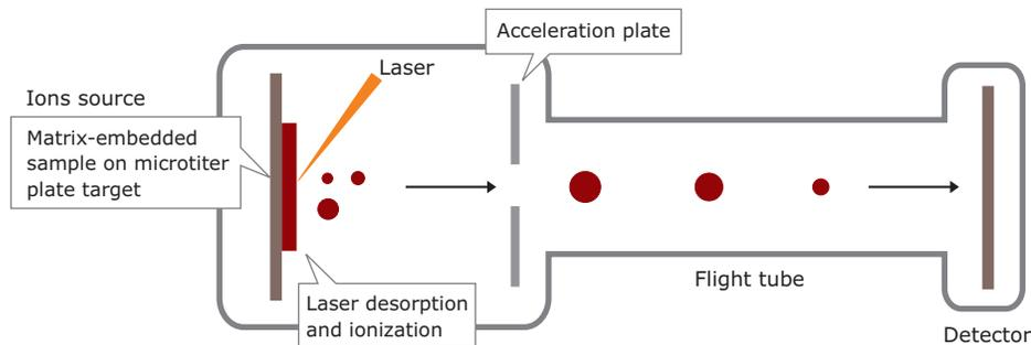
**Figure 4.3** Schematic representation of a MALDI/TOF mass spectrometer.
