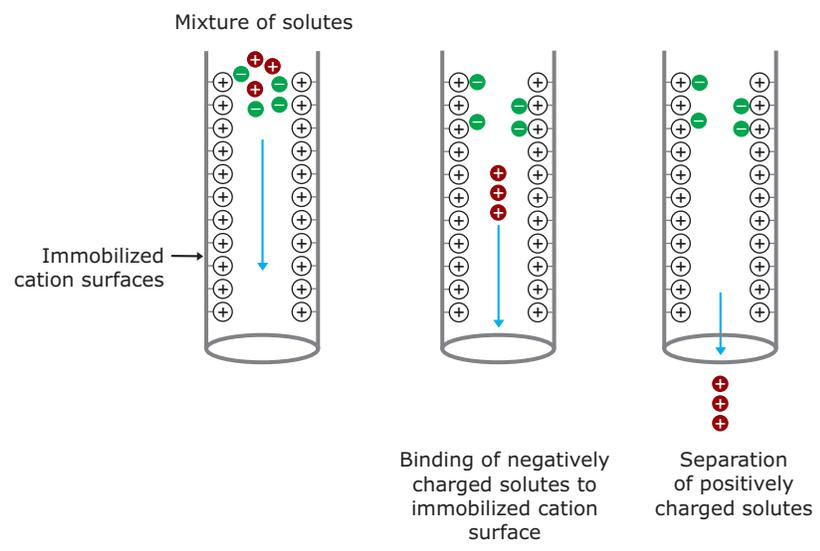
**Figure 1.4** Column materials used for ion exchange chromatography contain charged groups covalently linked to the surface of an insoluble matrix. The charged groups of the matrix can be positively or negatively charged. Anion exchangers have positively charged groups that will attract negatively charged anions. When a mixture of solutes is loaded into the anion exchanger, negatively charged solutes bind to the exchanger.
