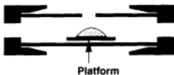
Figure 3.7 Isothermal operation using a platform.
