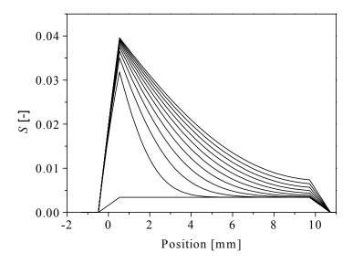
**Fig. 6.2.4-5** Simulated profiles with  $k_f = 1.92.10^{-7} \text{m.s}^{-1}$ . and constant diffusion coefficient  $D_{eff} = 5.61.10^{-11} \text{ m}^2 \text{s}^{-1}$ . Time between subsequent profiles is about 7 hours.
