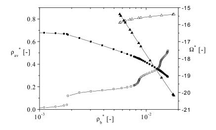
**Fig. 3.3-5a** Left vertical axis (open symbols): sorption isotherm, stable and metastable points. Right vertical axis (closed symbols): corresponding grand potential. The circles indicate the solution from the starting point at low adsorbate concentration. The squares indicate the filmlayer solution. The triangles indicate the solution from the starting point at high adsorbate concentration.  $w^*=10.49$ ,  $T^*=0.539$ .
