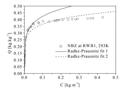
**Fig 2.4.3-1c** Sorption isotherms of nitrobenzene on AC RWB1 over wide concentration range. Fit 1 is Radke-Prausnitz fit of data points in fig. 2.3.4.1a. For fit 2 all data points were taken into account.
