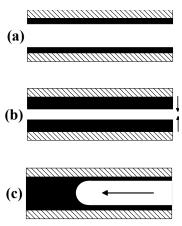
(a) Schematic representation of slit pore with one molecular Fig. 3.3.2-2 layer adsorbed at each pore wall. (b) Schematic representation of slit pore with growing of multiple molecular layers at each pore wall due to adsorption. (c) Schematic representation of slit pore with withdrawing capillary meniscus due to desorption. The first molecular layer at the pore wall remains.
