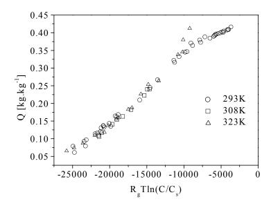
Fig 2.4.3-1b Potential plot of sorption isotherms of nitrobenzene on AC RWB1.
