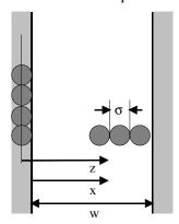
**Fig. 3.2.4-1** Schematic representation of a slit-pore with pore-width w, and molecular diameter  $\sigma$ .
