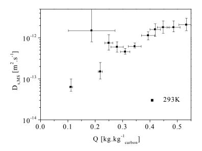
Fig. 5.5-2  $D_{s,MS}$  as a function  $Q_{NBZ}$  for AC R1-extra at 293K (nbz202).
