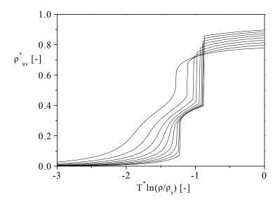
**Fig. 3.3-3** Isotherms from  $T^* = 0.77$  to  $T^* = 0.51$  (from left to right). Successive temperatures differ a factor 0.95.  $w^* = 4.26$ . The calculated isotherms with  $T^* > 0.79$  are not shown because in those cases the 2 components showed complete bulk miscibility (see figure 3.3-1).
