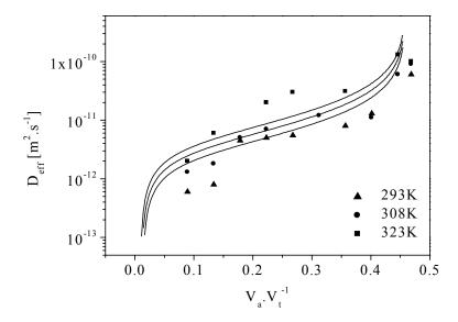
Fig. 4.3-2 Dependency of diffusivity of nitrobenzene on volume fraction filled with nitrobenzene at different temperatures. Comparison of the experimental data of Miyahara and Okazaki [1993] with  $D_{eff,I}$ , calculated by model I. F=0.0125.
