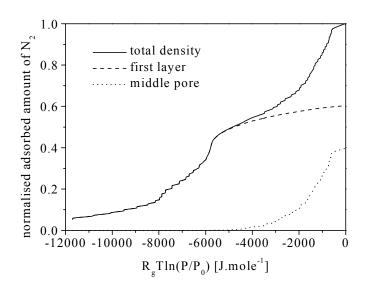
**Fig. 3.3.2-6b** Total isotherm (total density) of AC R1-extra, separated in part of adsorbate that is located in first molecular layer near pore wall (first layer) and adsorbate that is located in middle of pore, at least one molecular layer away from both pore walls (middle pore). Data from DFT calculations as in figure 3.3.2-3b.
