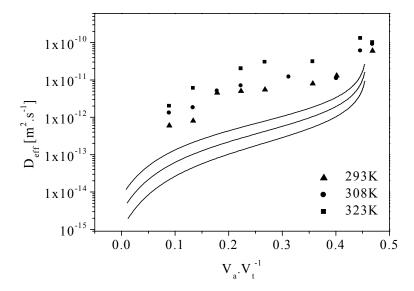
Fig. 4.1-2 Dependency of diffusivity of nitrobenzene on volume fraction filled with nitrobenzene at different temperatures. Comparison of the experimental data of Miyahara and Okazaki (1993) with  $D'_{w}$ , the contribution of molecular diffusion in the aqueous phase. Assumed is minimum tortuosity  $\tau$ =1.
