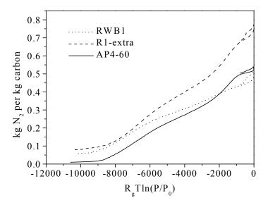
**Fig. 2.3.2-1** N<sub>2</sub> sorption isotherms at 77K for the activated carbons RWB1, R1 extra and AP4-60.
