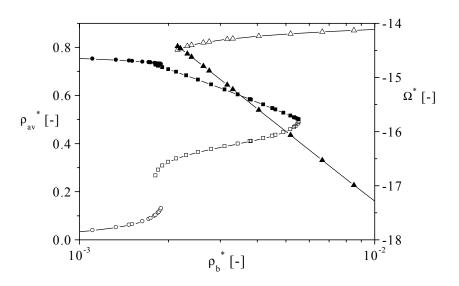
Fig. 3.3-2 Left vertical axis (open symbols): sorption isotherm, stable and meta-stable points. Right vertical axis (closed symbols): corresponding grand potential. The circles indicate the solution from the starting point at low adsorbate concentration. The squares indicate the film layer solution. The triangles indicate the solution from starting point at high adsorbate concentration.  $w^*$ =4.26,  $T^*$ =0.539.
