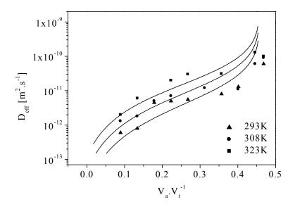
Fig. 4.3-4 Dependency of diffusivity of nitrobenzene on volume fraction filled with nitrobenzene at different temperatures. Comparison of the experimental data of Miyahara and Okazaki [1993] with  $D_{\it eff,II}$ , calculated by model II.  $\it F=1$ ,  $\it \delta=\delta_{min}+15$ .
