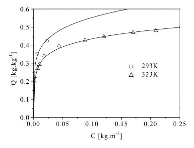
**Fig. 2.4.3-5a** Sorption isotherms of p-nitroaniline on AC R1-extra. The lines are the Radke-Prausnitz fits. Its parameters are given in table 2.4.3-1.
