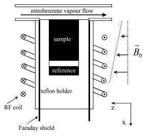
Fig. 6.1-3 MRI probe head with sample.
