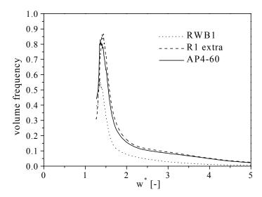
Fig. 3.3.2-5 Pore size distributions, calculated with the Horvath Kawazoe method from the N<sub>2</sub> sorption isotherm at 77K. (Derived from figure 2.3.2-2, under the assumption that the molar volume of N<sub>2</sub> inside the pores is constant)
