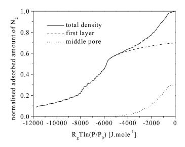
**Fig. 3.3.2-6a** Total isotherm (total density) AC RWB1, separated in part of adsorbate that is located in first molecular layer near pore wall (first layer) and adsorbate that is located in middle of pore, at least one molecular layer away from both pore walls (middle pore). Data from DFT calculations as in figure 3.3.2-3a.
