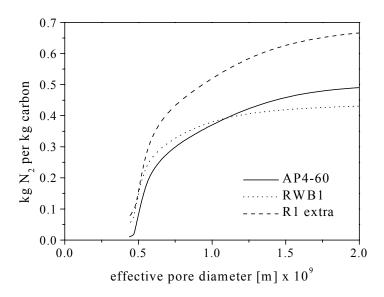
Fig. 2.3.2-2 Cumulative amount of nitrogen adsorbed as a function of pore size for the activated carbons RWB1, R1 extra and AP4-60, calculated with the Horvath Kawazoe method from the  $N_2$  sorption isotherms at 77K.
