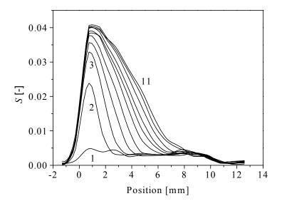
**Fig. 6.2.3-3b.** Profiles that have been normalised to the rubber reference signal. Data have been interpolated to equidistant time steps with a cubic spline. Time between subsequent profiles is about 7 hours. The sample is in contact with the nitrobenzene vapour flow at position x=0 mm.
