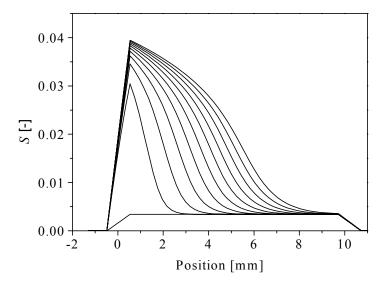
**Fig. 6.2.4-1** Simulated profiles with  $k_f = 0.569.10^{-7}$  m.s<sup>-1</sup> and a variable diffusion coefficient that is shown in figure 6.2.4-2. Time between subsequent profiles is about 7 hours.
