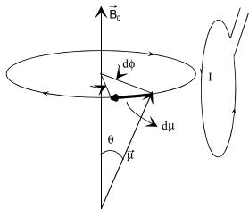
**Fig. 6.1-2** A precession movement of a nuclear spin induces an electrical current in a nearby coil.
