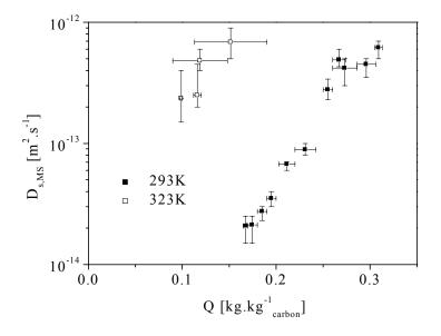
$\label{eq:problem} \begin{array}{ll} \textbf{Fig. 5.5-6} & D_{s,MS} \text{ as a function } Q_{QNX} \text{ for AC RWB1 at 293K } (qnx201) \\ & \text{and 323K } (qnx501). \end{array}$
