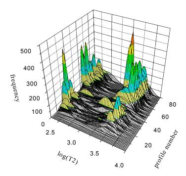
**Fig. 6.2.3-5**  $T_2$  distribution at position x=1.5 mm as a function of the profile number. The first profile denotes the start of the adsorption experiment. There are about fifty minutes between the subsequent profiles. The area under the curve at a certain profile number is proportional to the amount of protons (calculated with CONTIN [Provencher, 1982]).
