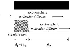
**Fig. 4.2.2-1** Schematic view of parallel capillary flow in adsorbate phase and molecular diffusion in aqueous phase, for discontinuous capillary flow (model II).
