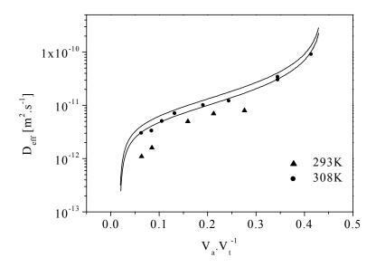
**Fig. 4.3-3** Dependency of diffusivity of benzonitrile on volume fraction filled with benzonitrile at different temperatures. Comparison of the experimental data of Miyahara and Okazaki [1993] with  $D_{eff,I}$ , calculated by model I. F=0.0125.
