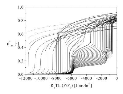
Fig. 3.3.2-1b Sorption isotherms of nitrogen at 77K calculated with DFT.
