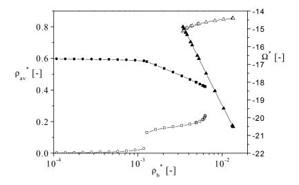
**Fig. 3.3-5b** Left vertical axis (open symbols): sorption isotherm, stable and metastable points. Right vertical axis (closed symbols): corresponding grand potential. The circles indicate the solution from the starting point at low adsorbate concentration. The squares indicate the filmlayer solution. The triangles indicate the solution from the starting point at high adsorbate concentration.  $w^*=10.49$ ,  $T^*=0.512$ .
