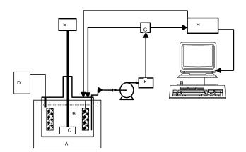
Fig. 5.2-1. Scheme of the experimental set-up for batch kinetic adsorption experiments, consisting of: a thermostated water-bath (A), batch vessel (B) with 2 baffles, 6-blade turbine stirrer (C,E), temperature recorder (D), filter holder (F), air-trap (G), UV\VIS spectrophotometer (H).
