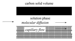
a fraction of the pores is filled with capillary liquid
