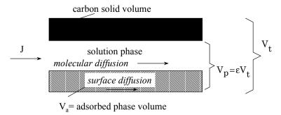
Fig. 4.1-1 Schematic representation of a model for parallel surface and molecular diffusion.
