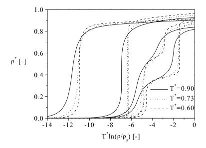
**Fig. 3.3.3-9** Case 6. Sorption isotherms at 3 different temperatures and 4 pore widths. Pore widths from left to right: 1.00, 1.82, 3.00 and 4.48 molecular diameters.
