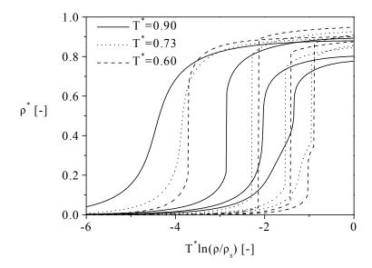
**Fig. 3.3.3-6** Case 3. Sorption isotherms at 3 different temperatures and 4 pore widths. Pore widths from left to right: 1.00, 1.82, 3.00 and 4.48 molecular diameters.
