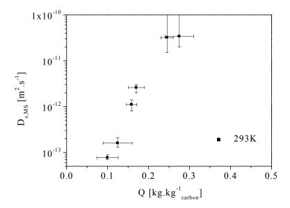
Fig. 5.5-3  $D_{s,MS}$  as a function  $Q_{NBZ}$  for AC AP4-60 at 293K (nbz203).
