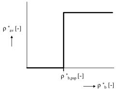
Fig. 3.3.3-10 Schematic representation of a sorption isotherm for a single pore. At bulk density  $\rho^*_{b,psp}$ , a capillary phase separation step
