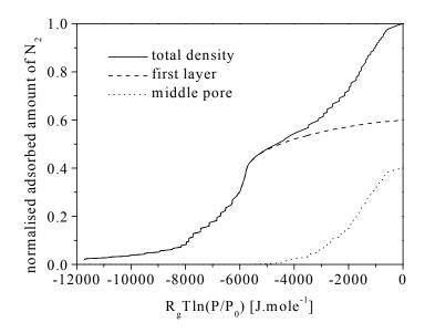
**Fig. 3.3.2-6c** Total isotherm (total density) of AC AP4-60, separated in part of adsorbate that is located in first molecular layer near pore wall (first layer) and adsorbate that is located in middle of pore, at least one molecular layer away from both pore walls (middle pore). Data from DFT calculations as in figure 3.3.2-3c.
