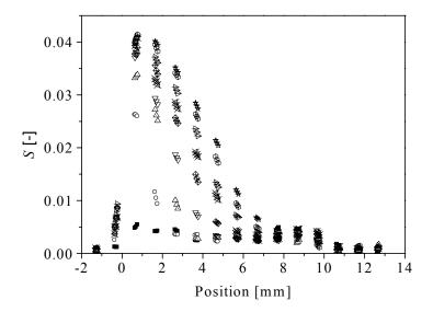
**Fig. 6.2.3-3a** Profiles that have been normalised to the rubber reference signal. The time between subsequent profiles is about 8.5 hours. The sample is in contact with the nitrobenzene vapour flow at position *x*=0 mm.
